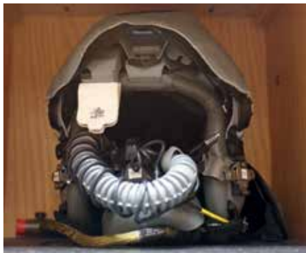
Above: Raytheon's Scorpion helmet technology transmits data via a monocle attached to an existing helmet to the pilot's right eye. Images by the authors unless stated otherwise
